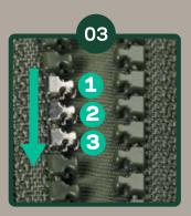
Attach additional replacement elements, one-by-one, next to the previously installed replacement element.
