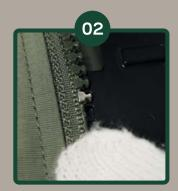
Attach first replacement element next to an undamaged VISLON® element.
