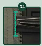
Align the plier jaw along the groove of the set plate.
